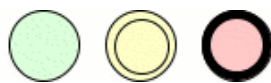
Figure B.2.: BPMN Event types. From left to right: Start Event, Intermediate Event, End Event
